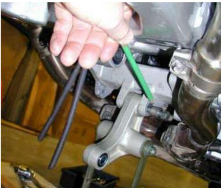
**The casting was very corroded and rarely past it's service life so a new one was required.** How much! Well if the old one is bugged I have to have a new one and bearings with a new pin. Thanks to my Son Chris who took the old casting to his work and had a tool made to press in the new bearings. I have some favours to repay and was the oven that mucky?
